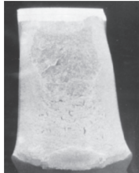
Figure CS3.10 Fracture surface of the Charpy impact specimen that was taken from the core region. [Reproduced with permission from Handbook of Case Histories in Failure Analysis , Vol. 1 (1992), ASM International, Materials Park, OH, 44073-0002.]
