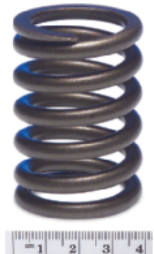
Figure CS2.4 Photograph of a typical automobile valve spring.
